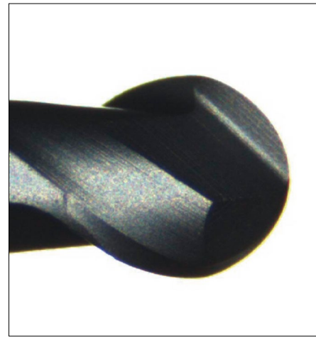
Diamond coated cutter diameter 0,10 mm under 750-fold magnification
