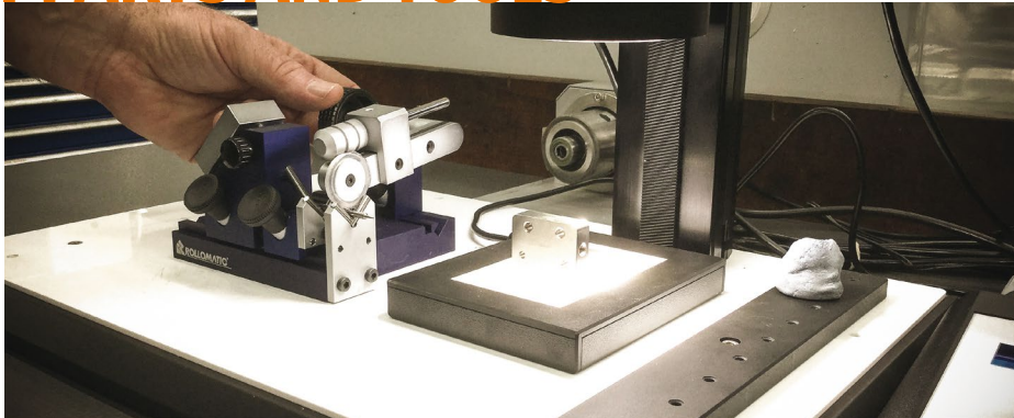
C-VIEW 500 with light and a high precision concentricity clamp
