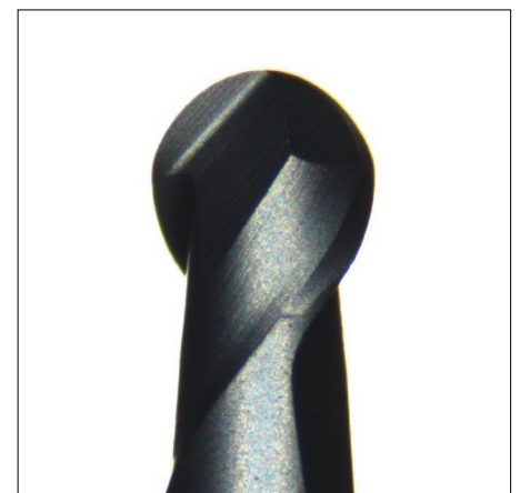
Ball cutter diameter 0,2 mm under 450-fold magnification
