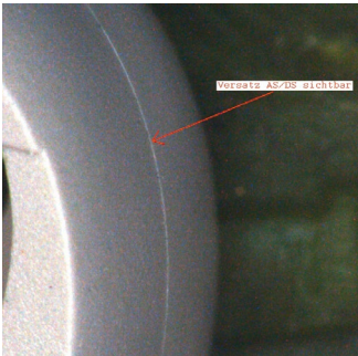
Misalignment on injection molded
