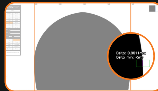
Automatic measurement of the tool runout
